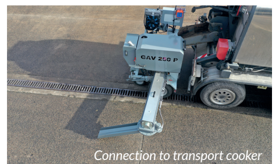
Operation of distributing arm
